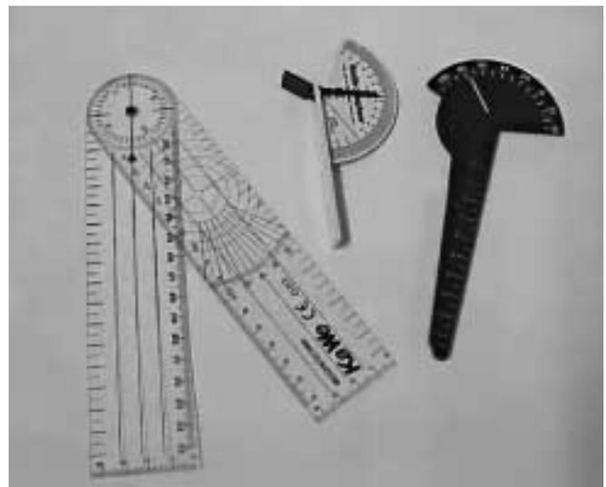
Figure 1.—Examples of conventional goniometers.
