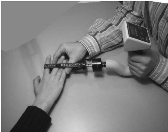
Figure 1. Illustration of the strength measurement of the abduction of the index finger using the Rotterdam Intrinsic Hand Myometer.
