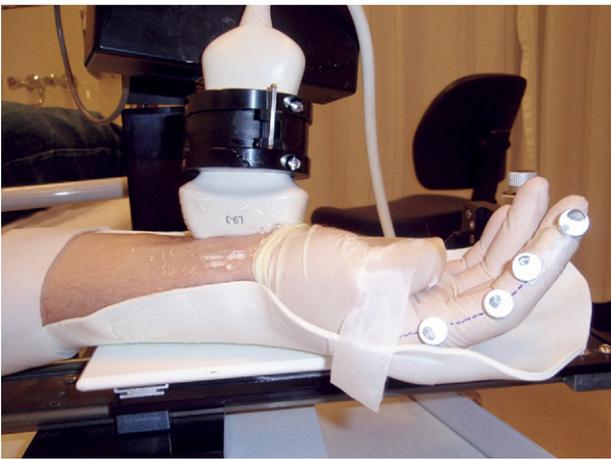
**FIGURE 1:** Experimental conditions with the subject's arm positioned in the custom-made brace. Four markers on the index finger were used to automatically track the joint angle.
